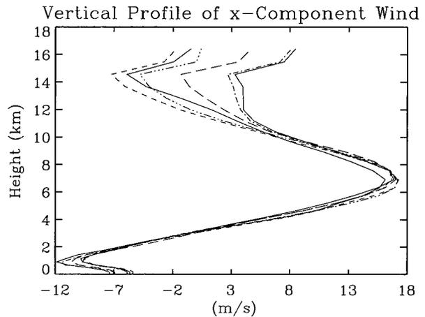
FIG. 2. Vertical profiles of domain-averaged  $x$ -component wind at every 10 h of simulation cM.
