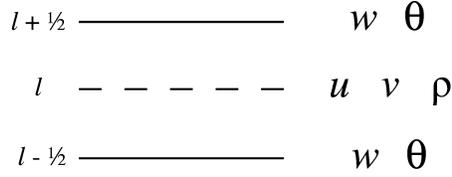
FIG. 1: Staggering of the prognostic variables on the vertical  $z$ -coordinate grid.
